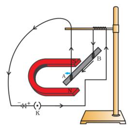
The displacement of the rod in the above activity suggests that a force is exerted on the current-carrying aluminum rod when it is placed in a magnetic field. Once the direction of field is changed to vertically downwards by interchanging the two poles of the magnet. The rod tends to move in the opposite direction. It shows that the direction of the force on the conductor depends upon the direction of current and the direction of the magnetic field.
